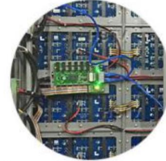
3. Connect power and signal cables.
