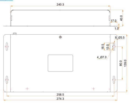
Tolerance: ±0.3 Unit: mm
